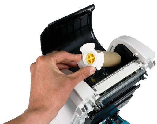
4. Install the paper core with **the right side first** onto the ribbon rewind hub first.
