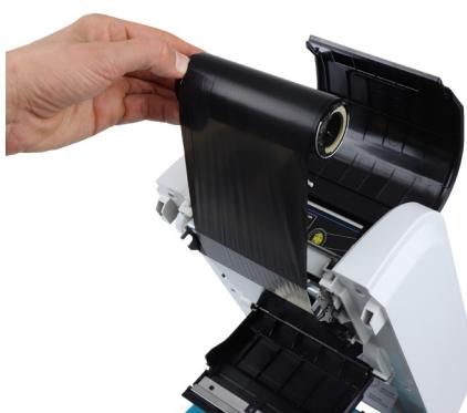
3. Remove the **waste roll** from the ribbon waste hub and place it on the ribbon supply cover.
