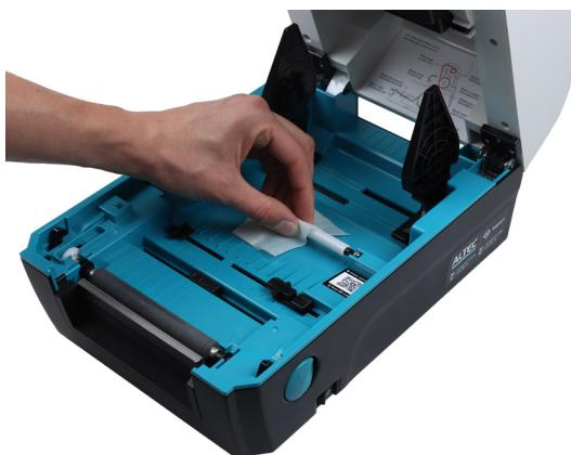
5. Clean the **media guide bar** and turn it around to clean it completely around.
