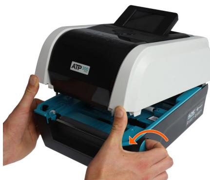
1. Open the top cover of the printer by pulling the **green levers** - located on each side of the printer - and lifting the top cover to the maximum open angle.
