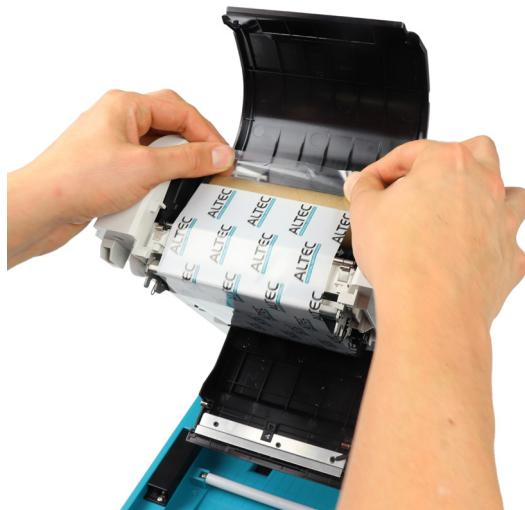
8. Turn the (waste) paper core with the (white) **ribbon rewind gear** until the plastic leader is thoroughly wound.
