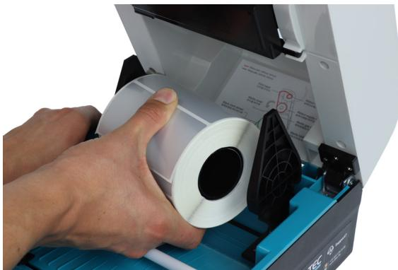
4. Place a roll of labels between the holders and close them onto the core.
