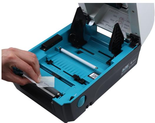
6. Clean the **platen roller** and turn it with both thumbs to clean it completely around.
