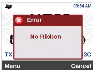
No ribbon installed or the ink ribbon has run out. [Go to chapter 3.2.](#)
