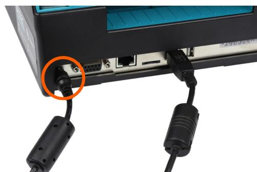
4. Plug the power cord into the **power cord socket** at the rear of the printer.
